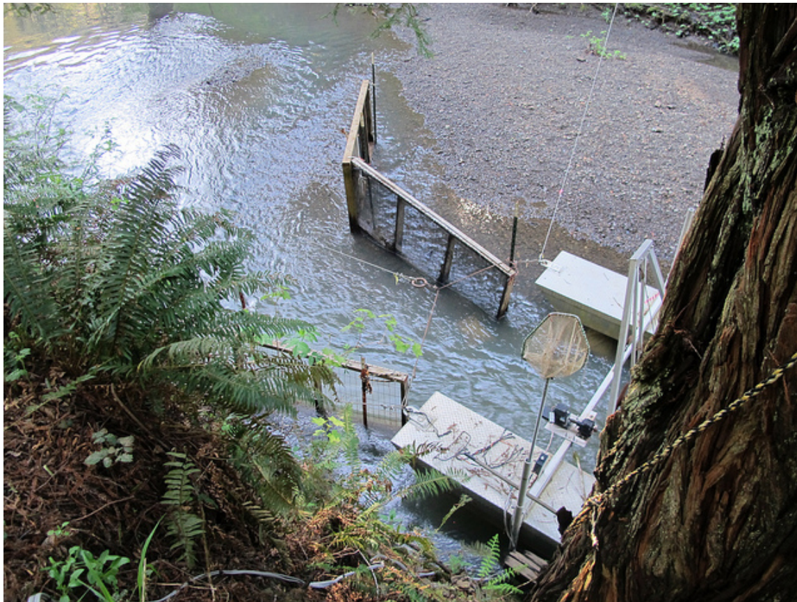
Figure 15. The Pudding Creek 5' rotary screw trap at low flows with the flow diversion panels.
