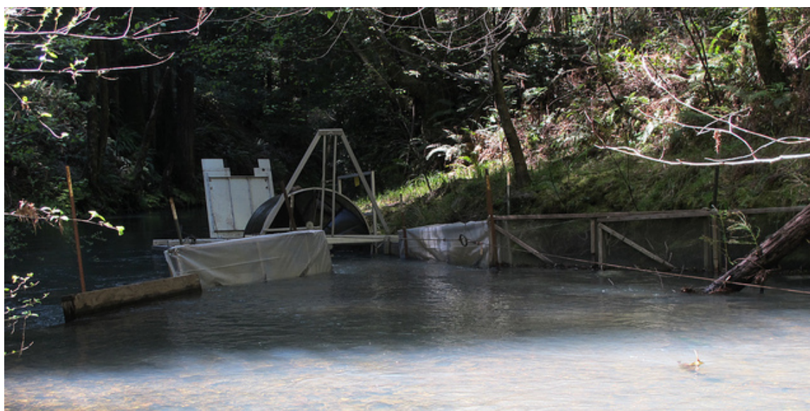
Figure 13. The Noyo River 5' rotary screw trap at low flows with diversion panels.
