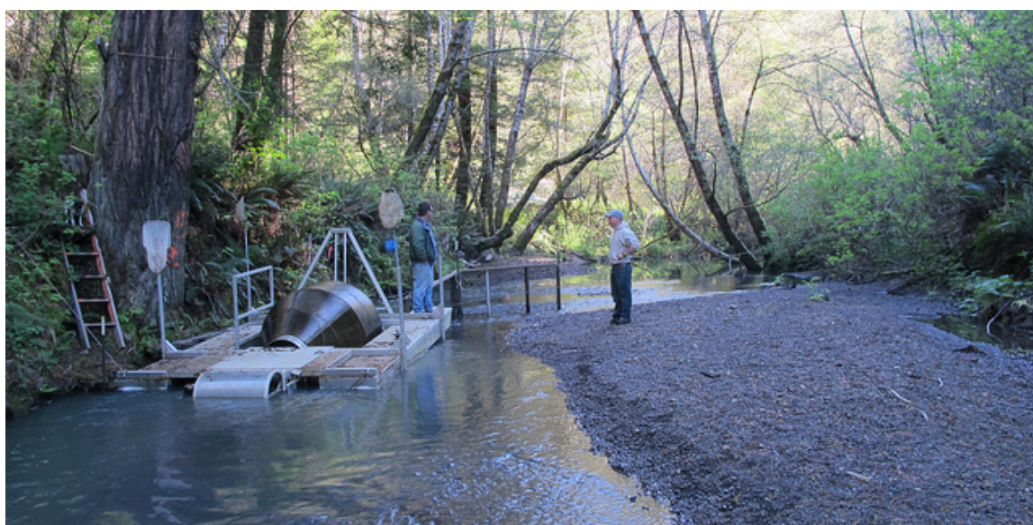
Figure 14. The Pudding Creek 5' rotary screw trap at low flows with diversion panels.
