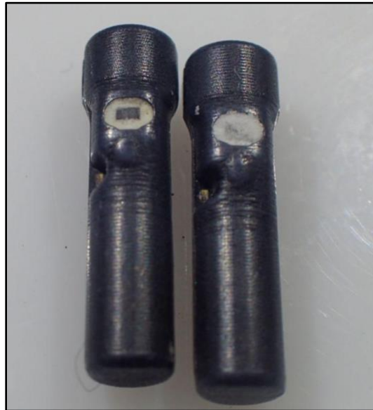
Figure 4. Example of a V3D tag that had been implanted in a juvenile rainbow trout for a period of three weeks (left), showing signs of corrosion of the trigger mechanism (not triggered), and a new transmitter showing an intact covering of the trigger mechanism (right).
