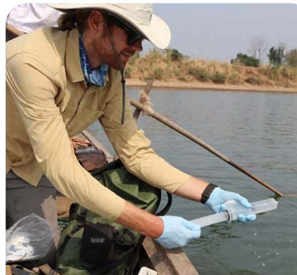
Water is pushed through a 5µm filter, which captures particles that may contain DNA.
